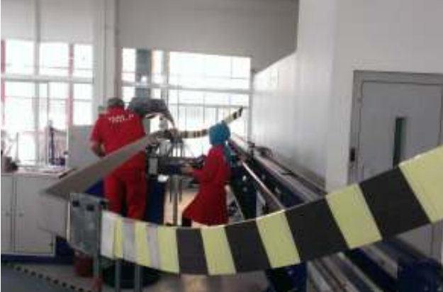
ROEBEL BAR SARGI İMALİ PRESSING ROEBEL BARS; FOR BIG GENERATORS PRODUCTION
